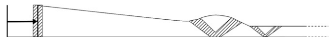
Fig. 12. Schematic cross-section for the experiments of prototypes 1A and 1B at the onset of the second thrusting event prior to the completion of experiments. The arrow shows the shortening and the shaded area illustrates the uncertainty for this shortening magnitude. The uncertainty for the positions and dips of the backthrusts and forethrusts is also shown with shading.
